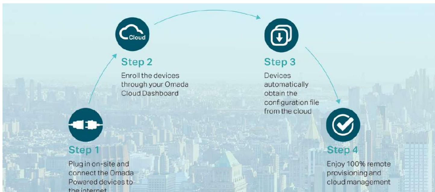
\* Zero-Touch Provisioning is supported when using Omada-Cloud Based Controller.
