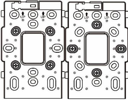
**Figure 3-4 Bracket on South African-standard 114 mm × 114 mm Junction Box**
