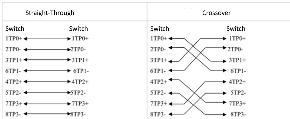
100BASE-TX/10BASE-T port can also be connected by cables of the preceding specifications. Besides, the 10BASE-T port can be connected by 100-ohm Category 3, Category 4, and Category 5 cables with a maximum distance of 100 meters (328.08 feet). 100BASE-TX port can be connected by 100-ohm Category 5 cables with a maximum distance of 100 meters (328.08 feet). The following table lists definitions of pin signals for the 100BASE-TX/10BASE-T port.
