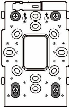
**Figure 3-5 Bracket on American-standard 108 mm × 59 mm Junction Box**
