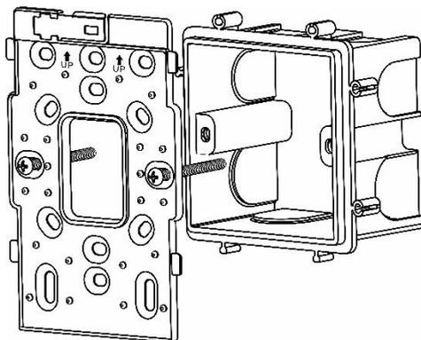
The following are brackets on European-standard 86 mm × 86 mm junction box, South African-standard 114 mm × 114 mm junction box, and American-standard 108 mm × 59 mm junction box. The access point can be mounted horizontally or vertically on a South African-standard junction box.
