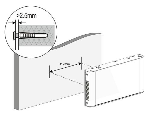
RG-ES126G-P-L is provided with mounting brackets. The installation process is as follows:
