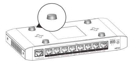
Figure 3-8 Attaching the Rubber Pads to the Recessed Areas
