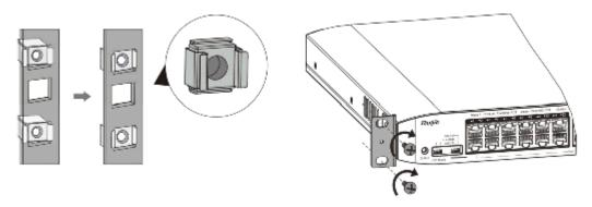
Figure 3-3 Attaching the Brackets to the Rack to Install RG-ES126G-P-L
