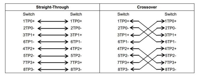
In addition to the above cables, the 100BASE-TX/10BASE-T can also use 100-ohm Category-3, 4, 5 cables for 10 Mbps, and 100-ohm Category-5 cables for 100 Mbps, both of which can be up to 100 m. 0 shows the pinouts of the 100BASE-TX/10BASE-T.
