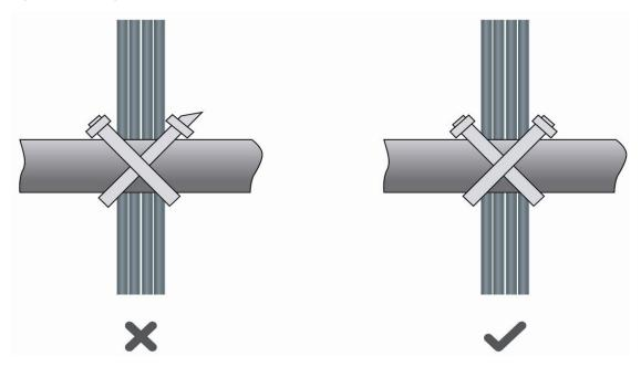
• If cables are to be bent, bind them first but do not tie cable ties within the bend to avoid stress on the cables, which may otherwise cause the wires inside to break, as shown in Figure D-3.
