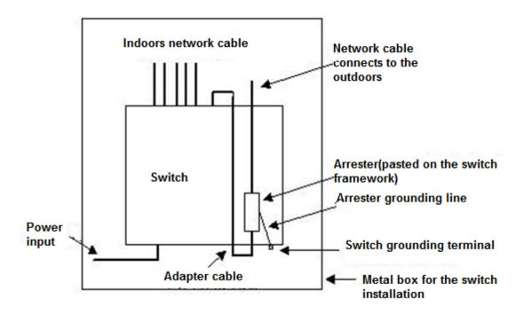
The Ethernet port arrester is only for the 10M/100M copper Ethernet ports with the RJ-45 connector;
