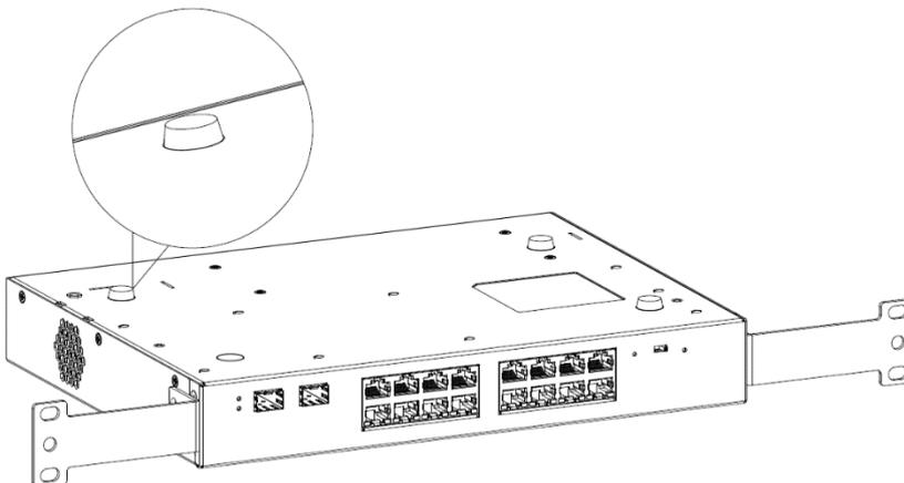
Figure 3-8 Attaching the Rubber Pads to the Recessed Areas
