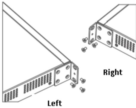
Step 2: Use the supplied M6 screws and cage nuts to securely attach the mounting brackets to the rack, as shown in Figure 3-4 and Figure 3-5.
