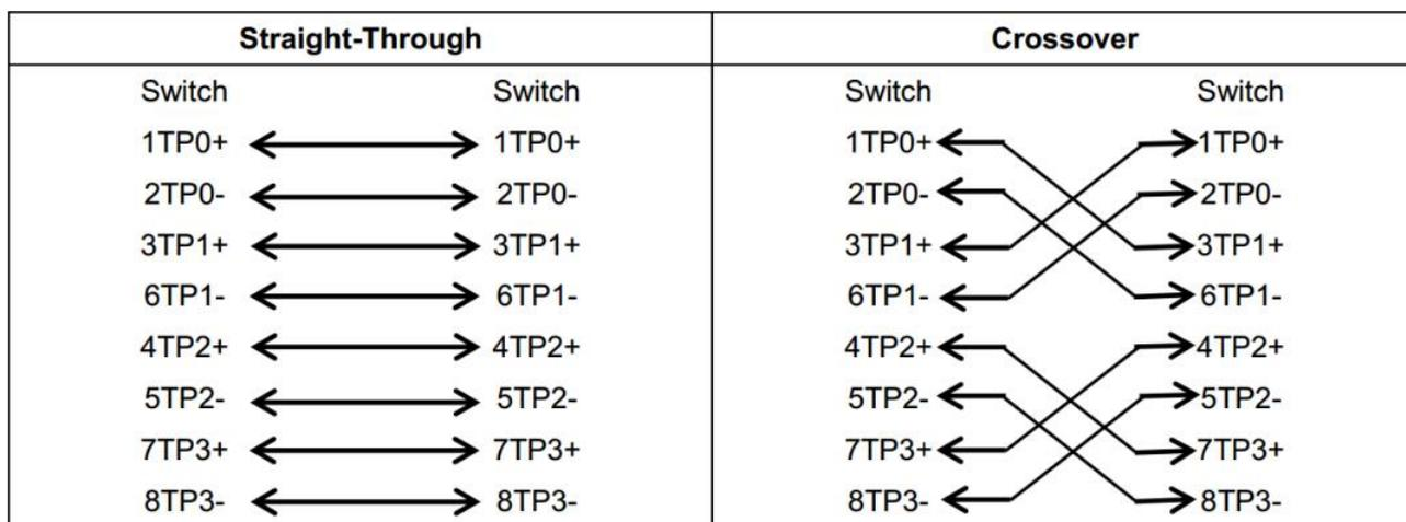
In addition to the preceding cables, the 100BASE-TX/10BASE-T can also use 100-ohm Category-3, 4, 5 cables for 10 Mbps, and 100-ohm Category-5 cables for 100 Mbps, both of which can be up to 100 m. Figure A-2 shows the pinouts of the 100BASE-TX/10BASE-T.
