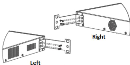
Figure 3-2 Attaching the Mounting Bracket to the RG-ES226GC-P
