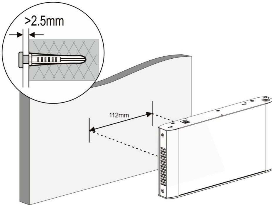
RG-ES126G-P-L is provided with mounting brackets. The installation process is as follows:
