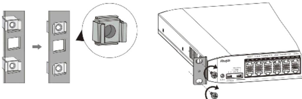
Figure 3-3 Attaching the Brackets to the Rack to Install RG-ES126G-P-L
